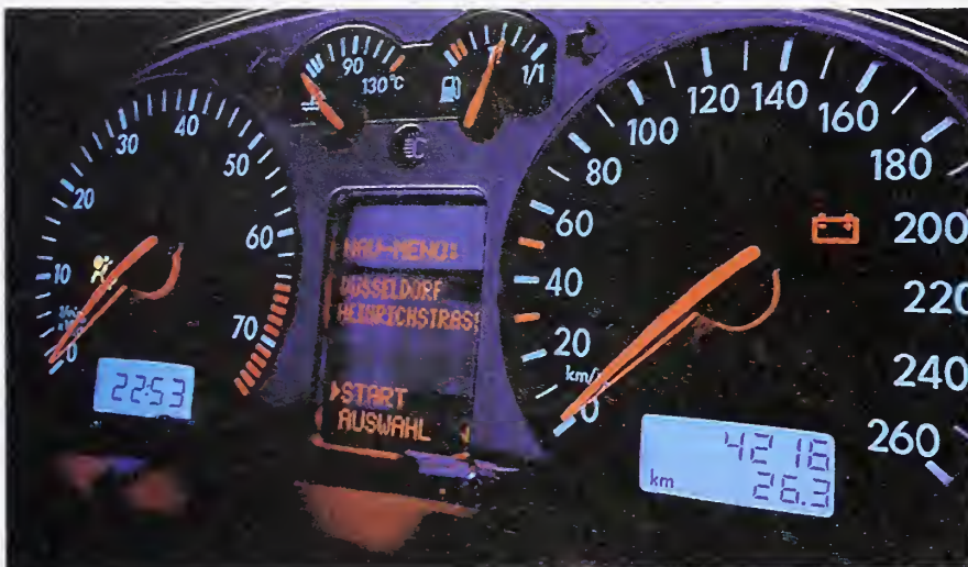
Cree's LED chips are used by Siemens A.G. for back lighting for this dashboard.
